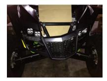
6. Disconnect the headlight plugs (2 each side). Locate the headlight adjuster knob on the inboard side of both headlights and remove. Now, using the needle-nose pliers, remove the four silver retaining clips on each of the headlight mounting points.
