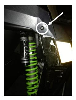
4. Now, at the front of the vehicle, locate the two pressed in black plastic fasteners near the front corners of the hood opening that secure the grill. Using a standard screwdriver, pry up the center section until it appears as shown below.
