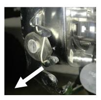
7. For the driver side, it will require removal of the headlight subframe. Gently work the outboard headlight mount until it is almost able to be slid out. Remove two T30 bolts per side of the subframe bracket. As the bracket is being removed, support the headlight and carefully demount the light from the subframe. Now, remove the headlight.
