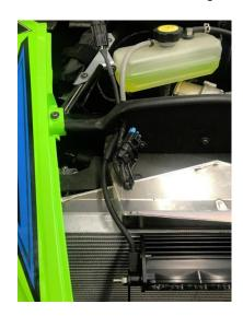
15. If you have purchased the additional Baja Designs Textron Wildcat Headlight kit (44-7094, 44-7095, 44-7096), skip steps 15-16. Now it is time to remount the stock headlights. Beginning with the passenger side, place it into the opening as shown below. Align the headlight mounts and the tilt adjuster assembly simultaneously. It may be necessary to bend the U-bracket slightly for the next step.
